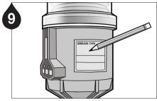
Note the installation date and the scheduled completion date of lube cycle on the lubricator using the label provided in the Service Pack for maintenance purposes.
