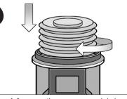
Carefully screw the grease pouch in by turning clockwise. Do not over tighten.
