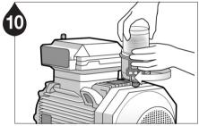
Install the Lubri-Cup EM unit on the lube point. When the selected dispensing period has completed, replace the Service Pack following steps 3~6.
