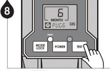
Press the **TEST** button for 2 seconds to run a test cycle and check for proper operation of the unit.
