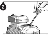
Ensure a clear passage using a manual grease gun. Note1 Remove any hardened grease by purging the lube point with a manual grease gun. Note2 The grease in the equipment and the grease contained in the unit should be the same or compatible
