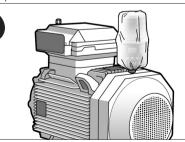
Install the dust cover over the lubricator for added protection.
