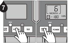
Press **POWER** button for 2 seconds to power on. Press **MODE** button to select dispensing period.
