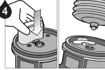
Insert battery pack and purge the grease pouch until grease comes out of the tip.
